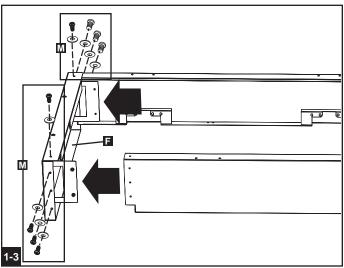
Insert the upper end of the left and right vertical sections into the top section **E**. Align the screw holes, insert eight M5 x 10 mm screws and washers **M** and tighten securely. (Start all the screws before tightening.)
